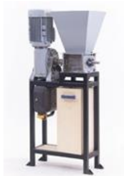
Picture 31. Machine built from Precious Plastics for recycling plastic
